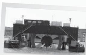
A turbine is being put in the ocean near a tidal power plant. The water pushes the turbines, and it spins. This is how the energy is moved from the ocean to the power station.
